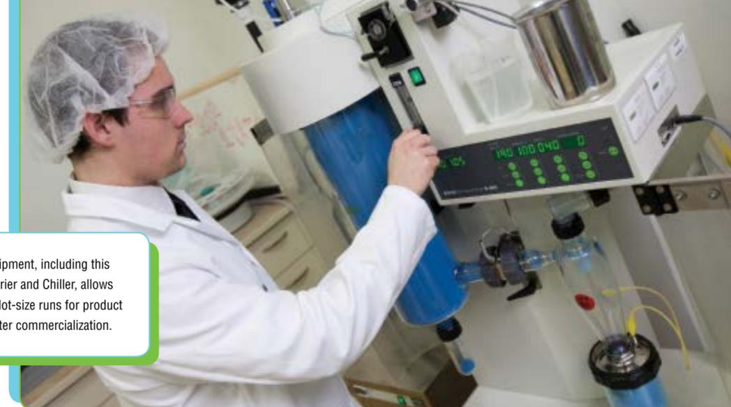
FONA's in-house equipment, including this Büchi B-290 Spray Drier and Chiller, allows quick and efficient pilot-size runs for product development and faster commercialization.
